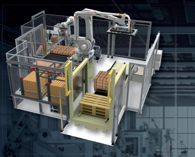
The palletization island is designed and built to palletize diaper boxes and wrap completed pallets.
