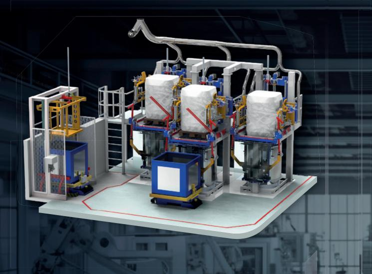
The AGM AUTOMATIC LOADING SYSTEM has been designed to automatically perform the loading operations of AGM bags into the silos, which supply Baby Care production lines.
